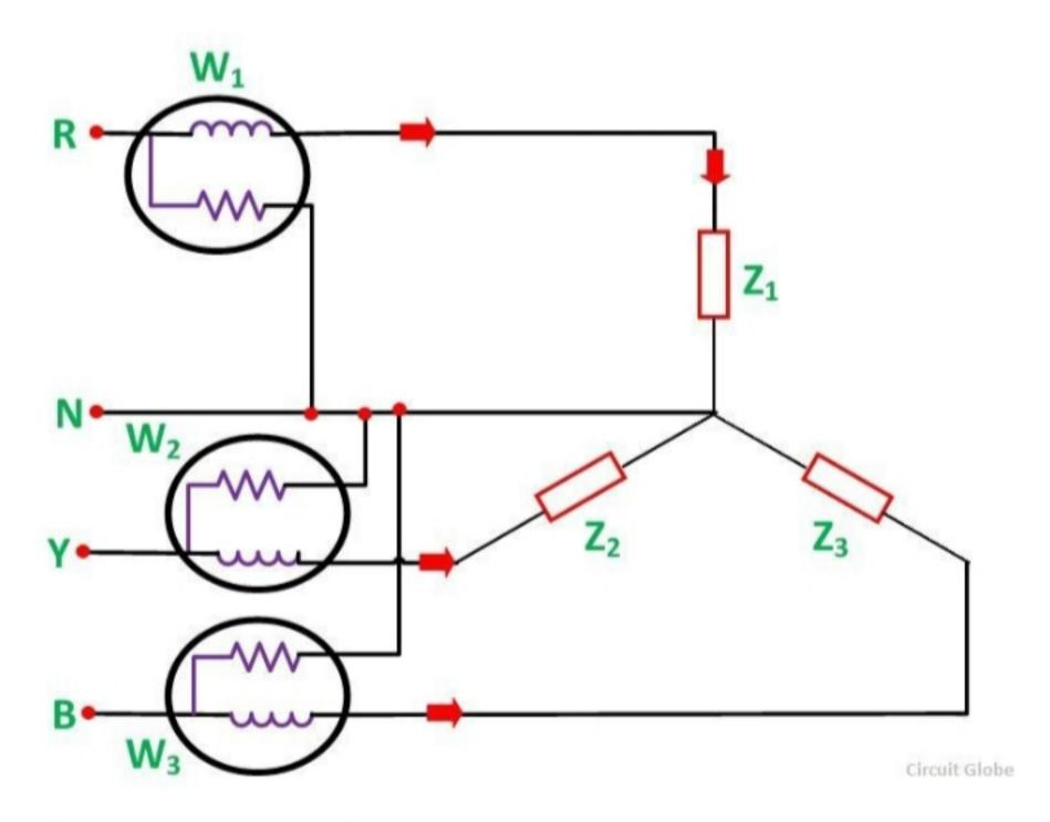
The pressure coil of all the three wattmeters namely  $W_1$ ,  $W_2$  and  $W_3$  are connected to a common terminal known as the **neutral point**. The product of the phase current and line voltage represents phase power and is recorded by an individual wattmeter.
