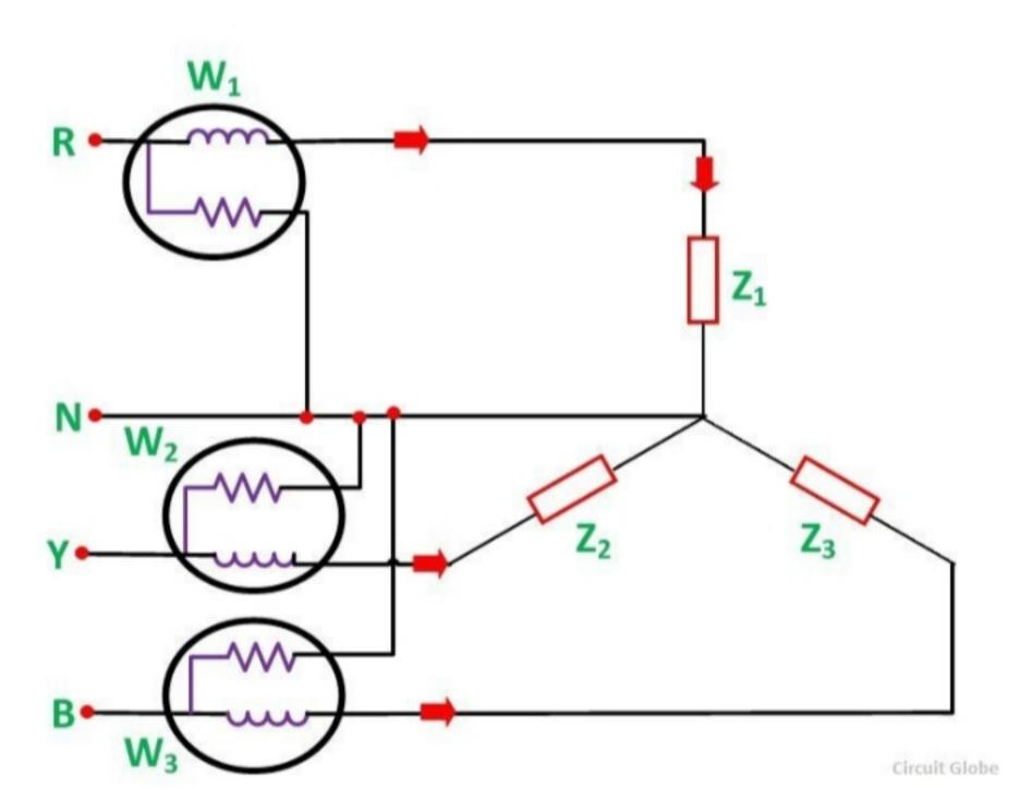
The connections for star connected loads for measuring power by three wattmeter method is shown below:
