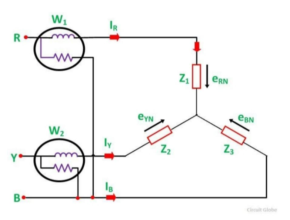
The total instantaneous power absorbed by the three loads Z<sub>1</sub>, Z<sub>2</sub> and Z<sub>3</sub>, is equal to the sum of the powers measured by the two wattmeters, W<sub>1</sub> and W<sub>2</sub>.
