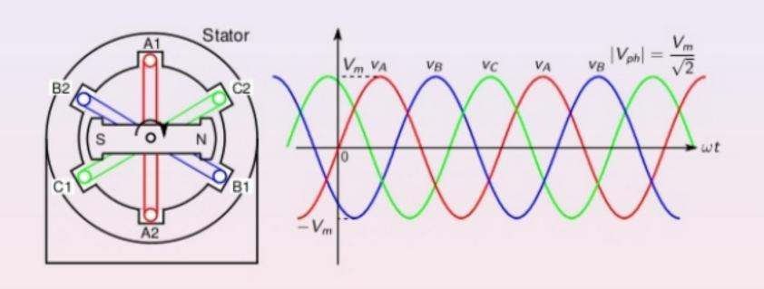
$$v_A = V_m \sin \omega t \implies V_A = |V_{ph}| \angle 0^\circ$$
