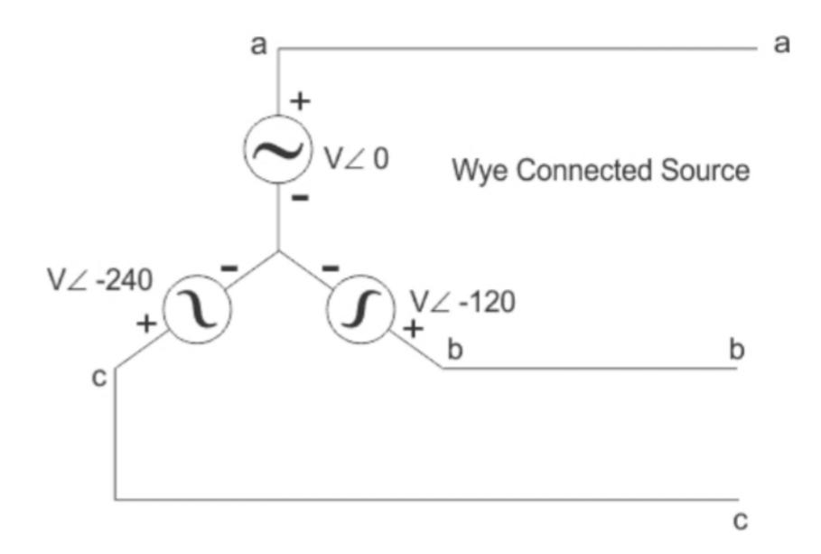
In star connection, the line voltage is √3 times of phase voltage. Line voltage is the voltage between two phases in three phase circuit and phase voltage is the voltage between one phase to the neutral line. And the current is same for both line and phase. It is shown as expression below
