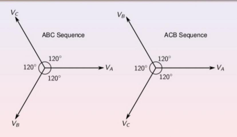
Phase sequence can be changed by reversing the direction of rotation of rotor of the alternator.
