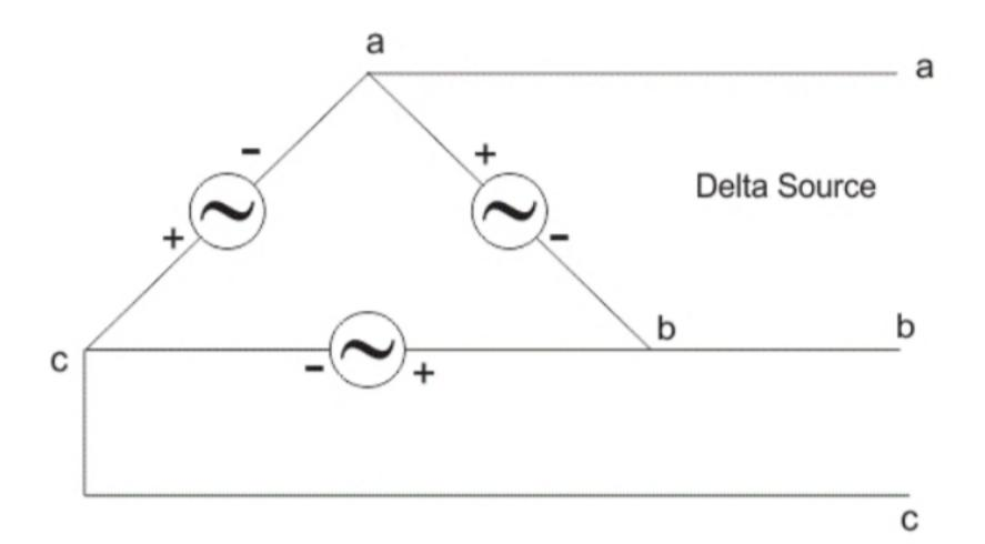
In delta connection, the line voltage is the same as that of phase voltage. And the line current is √3 times of phase current. It is shown as expression below,
