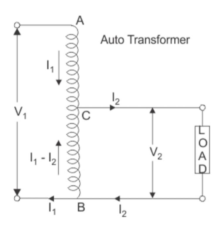
The winding AB of total turns  $N_1$  is considered as primary winding. This winding is tapped from point 'C' and the portion BC is considered as secondary. Let's assume the number of turns in between points 'B' and 'C' is  $N_2$ .
