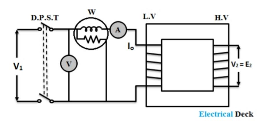
Sometimes, a high resistance voltmeter is connected across secondary to read secondary induced emf which helps to find the transformation ratio K.
