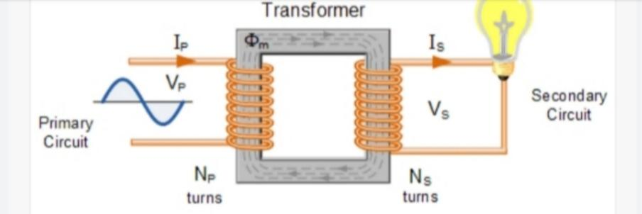
In other words, for a transformer there is no direct electrical connection between the two coil windings, thereby giving it the name also of an **Isolation Transformer**. Generally, the primary winding of a transformer is connected to the input voltage supply and converts or transforms the electrical power into a magnetic field. While the job of the secondary winding is to convert this alternating magnetic field into electrical power producing the required output
