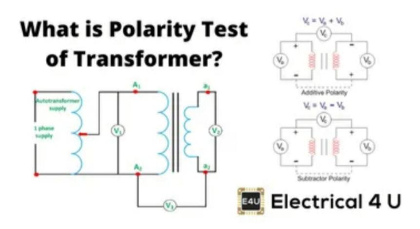
Current flows from high voltage point to low voltage point due to the potential difference between them. Here, electrical polarity comes into the picture. Electrical polarity simply describes the direction of the current flow. When we look into DC system, we find that one pole is always positive and
