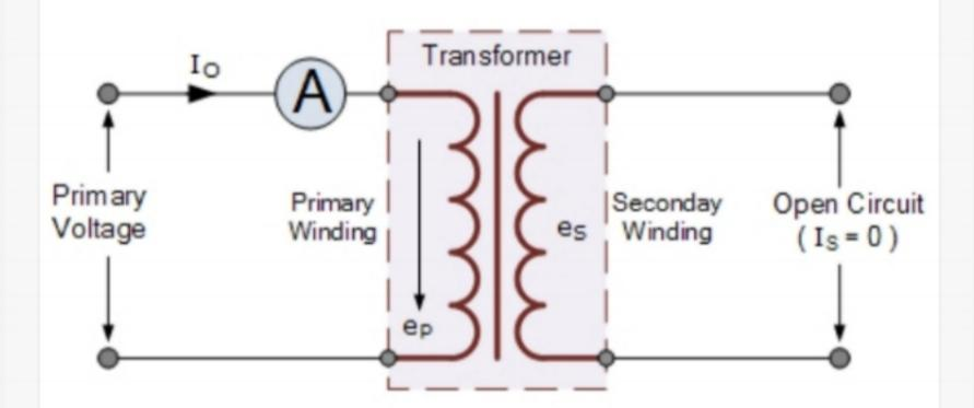
The ammeter above will indicate a small current flowing through the primary winding even though the secondary circuit is open circuited. This no-load primary current is made up of the following two components:
