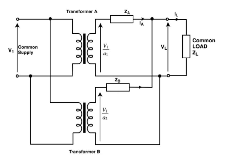
Fig: Two single-phase transformers in parallel.
