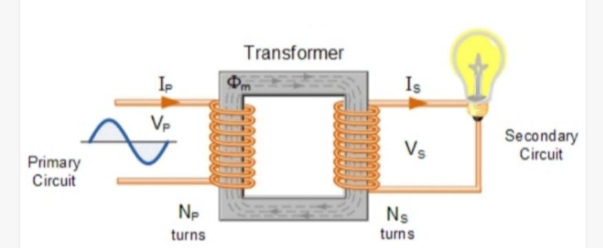
In other words, for a transformer there is no direct electrical connection between the two coil windings, thereby giving it the name also of an **Isolation Transformer**. Generally, the primary winding of a transformer is connected to the input voltage supply and converts or transforms the electrical power into a magnetic field. While the job of the secondary winding is to convert this alternating magnetic field
