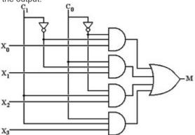
The diagram of a 4-to-1 multiplexer is shown below:
