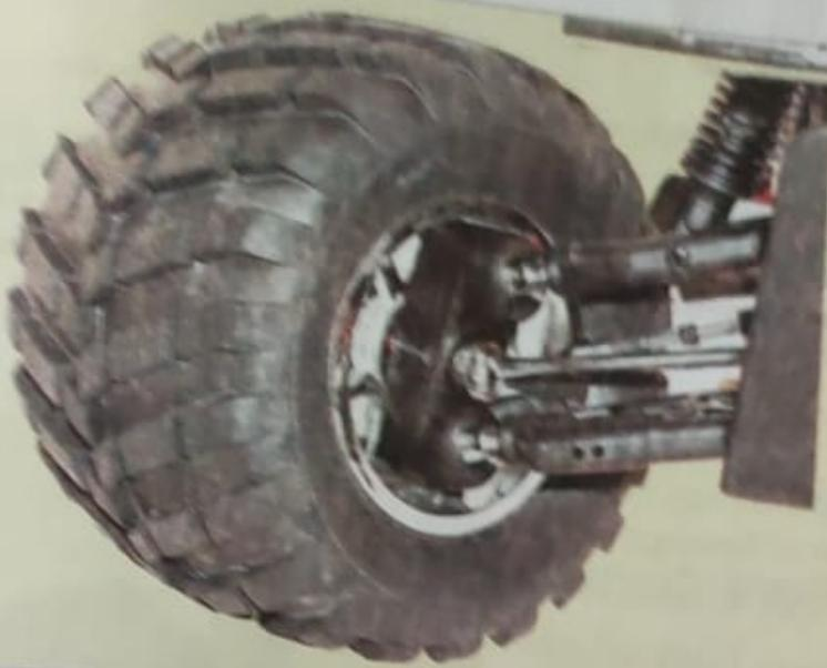
**Front suspension system:** Front Pivot ball suspension soaks up the bumps and provides unmatched adjustability. Chrome 8 mm CVA joints give added strength.
