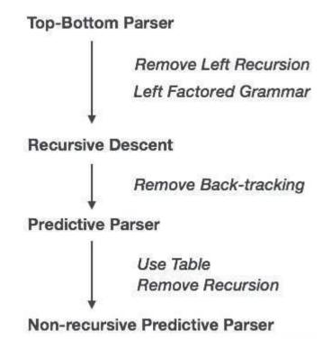
In recursive descent parsing, the parser may have more than one production to choose from for a single instance of input, whereas in predictive parser, each step has at most one production to choose. There might be instances where there is no production matching the input string, making the parsing procedure to fail.
