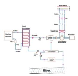
**Nuclear reactor.** It is an apparatus in which nuclear fuel  $(U^{235})$  is subjected to nuclear fission. It controls the chain reaction that starts once the fission is done. If the chain reaction is not controlled, the result will be an explosion due to the fast increase in the energy released.
