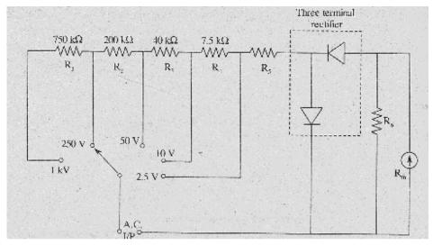
fig 9.1 Multi Range A.C Voltmeter
