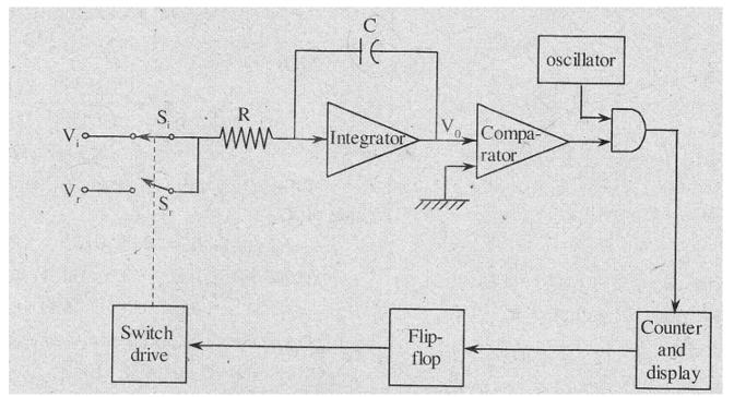
fig 10.1 Block Diagram of Dual slope integrating Type DVM
