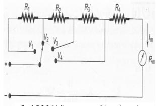
fig 4.3 Multiplier connected in series string
