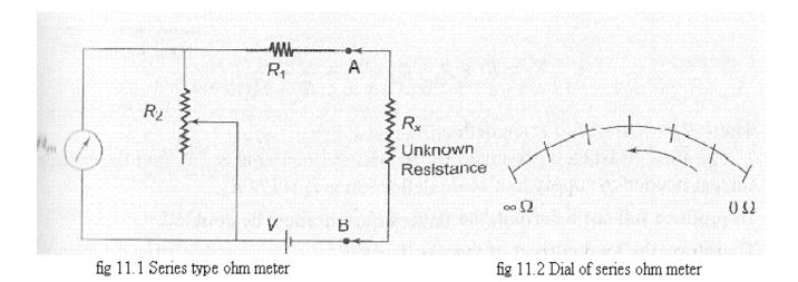
The current flowing through the movement then depends on the magnitude of the unknown resistance. Therefore, the meter deflection is directly proportional to the value of the unknown resistance referring to the figure 11.
