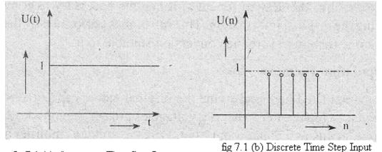
fig 7.1 (a) Continuous Time Step Input
